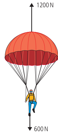
Figure 2.74 The parachutist just after opening the parachute.
